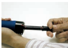
3. Align the guide marks for the desired sample size, then pull the pump handle.
