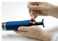
1. Break the glass tips off both ends of the detector tube.
