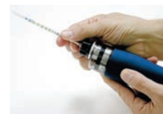
2. Insert tube into the pump inlet with the arrow on the tube pointing toward the pump.
