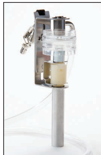
NIOSH 0600 requires use of a Dorr-Oliver Cyclone. See Dorr-Oliver Cyclone on page 39.
